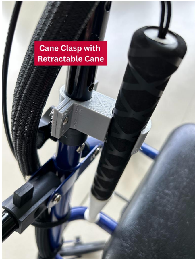
Figure 13. Smart Autonomous Rollator (SAR) - Cane Clasp with retractable cane
